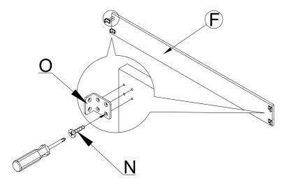
4. Attach the Side panel (F) to the Headboard (A), under the Side rail (D) using 4pcs Phillips head screws 7x20mm (N) as shown. Repeat the same procedure with the Footboard (B).
