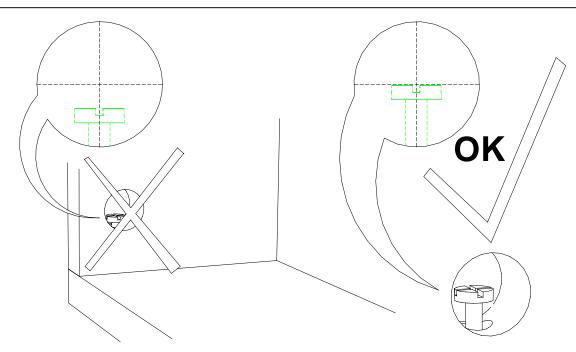
2. Using (1) Wooden Connector Pin (E) fasten (1) Long Side Rail to the Bottom Board.
