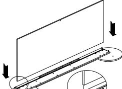
3. Insert (2) Short Side Rail over the Cam Both Sticking out of the Long Side Rail.
