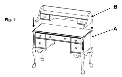
2. Secure the hutch (B) to the desk (A) by assembling the mending plates (C) into the pre-drilled holes on the back of the hutch and desk using screws (D). Tighten using a Phillips head screwdriver, as shown in fig. 2
