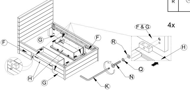
6. Adjust the lever(up and down) on (H) . as shown below.
