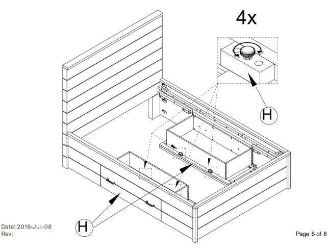
7. Attach (I)to (H). as shown below. Check alignments and secure all bolts with (K). Ν 8x Q 8x (H) R 8x
