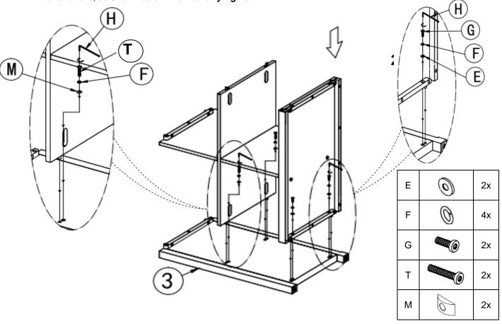
4. Attach (4) to the assembled pieces by aligning the pre-drilled holes with the wooden dowels and secure with the hardware, as shown below. **Do not fully tighten.**
