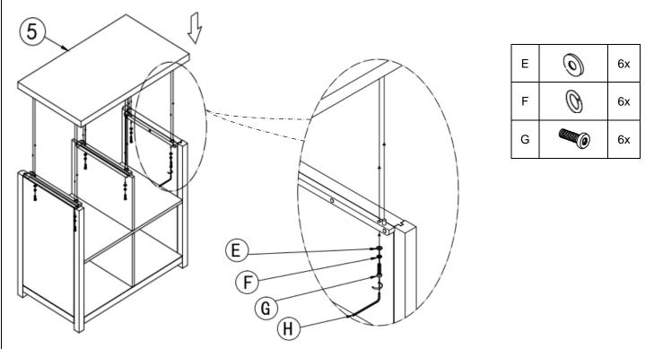
6. Check alignments and fully tighten all connections at this time. Do not over tighten.
