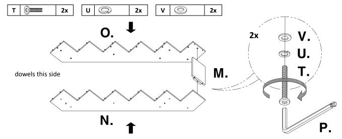
2. Attach the Stair Landing (K) onto wooden dowels located on the other ends of the Left/Right Wall String (N&O). Insert (2) Short Bolts (T) with washers to secure. Do not fully tighten.
