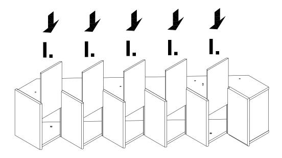
5. Align pre-drilled holes to attach the assembled stair unit to the Ladder Right Side (B). Insert (6) Short Bolts (T) with washers from pre-drilled holes on the assembled stair unit into pre-drilled holes located on the Ladder Right Side (B) to secure but do not over tighten.
