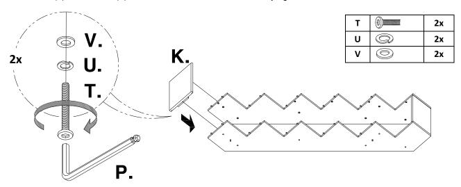
3. Attach the First Tread (L) and remaining(4) Tread (J) onto wooden dowels located on the Left/Right Wall String (N&O) as shown. Insert (2) Short Bolts (T) with washers to secure each tread to the wall strings. Do not fully tighten.
