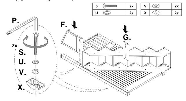
7. Attach Ladder Left Side (E) onto the assembled piece. Insert Medium Bolt (S) with washer (U)&V) and Half-Moon Metal Block (X) from cut-out on the Ladder Back into pre-drilled holes on the Ladder Left Side (E).
