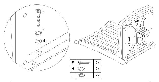
Date: 2012-Jun-30 Rev: 2013-Dec-02 5. To attach the assembled seat to the Chair Base (C), align and connect the hole in center of the Metal Bracket at bottom of the Chair Seat onto the assembled Cylinder (J) on the Chair Base. Firmly apply pressure onto the Chair Seat with both hands to ensure chair slides onto the Cylinder (J). Use Allen Key to tighten the pre-installed bolt against the cylinder as seen in illustration below.
