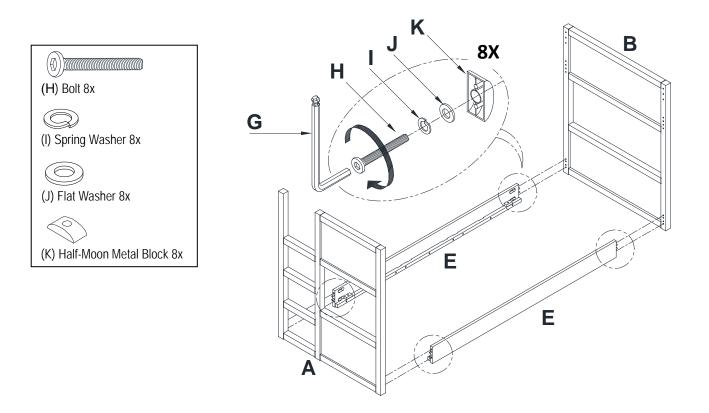
3. Attach (1x) Upper Side Rail (D) to the assembled piece by aligning wooden dowels on the side rail to pre-drilled holes on the Front Gate Panel and Back Panel. Secure the side rail using 4 sets of: Spring Washer (I), Flat Washer (J), Half-Moon Metal Block (K) and Bolt (H), as shown in the illustration below. Tighten by Allen Key (G). Do not fully tighten the bolts.
