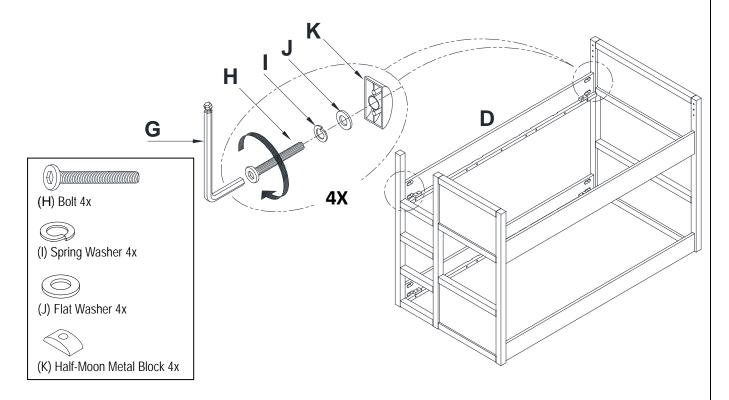
5. Attach (2x) Guardrail (C) to the assembled frame by aligning wooden dowels on the guardrails to pre-drilled holes on the Front Gate Panel and Back Panel. Secure the Guardrail © using 4 sets of: Spring Washer (I), Flat Washer (J), Half-Moon Metal Block (K) and Bolt (H), as shown in the illustration below. Tighten by Allen Key (G). Do not fully tighten the bolts.
