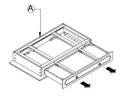
3. Attach Left side panel (B) to Top Panel with Drawer (A) with Allen Bolts 1/4"x25x13mm (G), Spring Washers 1/4"x10x1.5mm (H) and Flat Washers 1/4"x12x1.5mm (I) as shown below, tighten by the Allen Key with ball tip (F).
