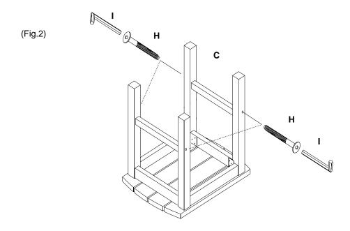
3. Tighten all nuts and bolts. Turn the piece upright. Assembly is complete
