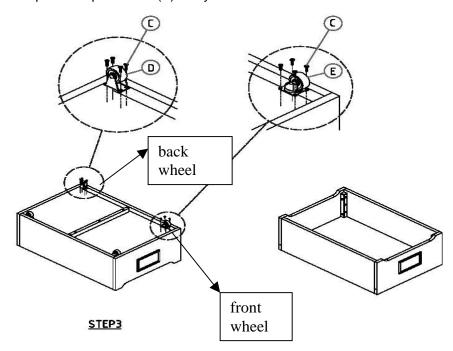
3. Turn the Cart upside down on a soft surface. Attach swivel castors (E) in the front, fixed wheel castors in the back of the cart, then tighten up with Phillips screws (C) using screw driver (not included).
